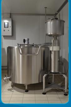
For faster cooling and important energy and water saving, the icebank system is optionally provided.
