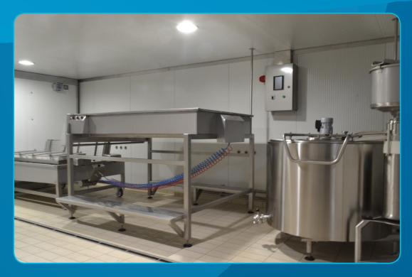
**MP CheeseMaker by Milkplan** is a complete cheese production line for milk capacity from 100 to 500 liters. It is a reliable and functional solution for small and flexible units.
